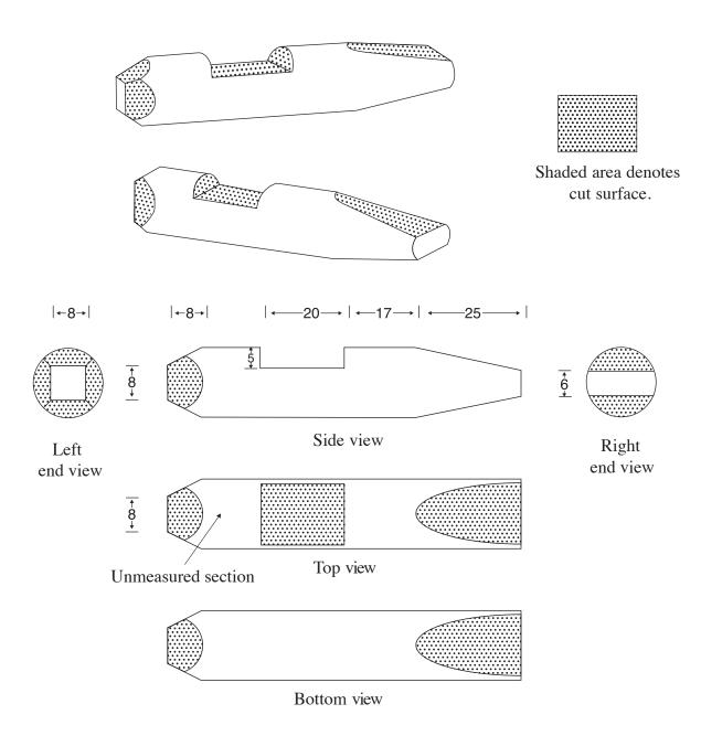
All measurements shown in millimetres
